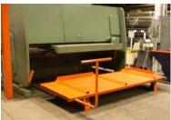
← Building a cart and rail system for the shear reduced the time to retrieve parts and
